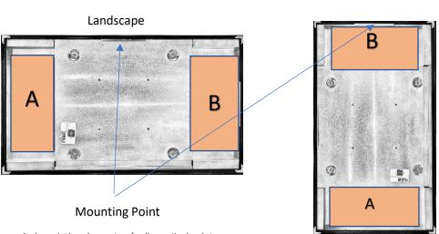
Anchor point based on center of wall mounting bracket (Measurements assume you are using Nimbus Supplied wall mount)
